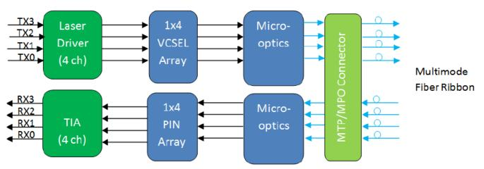
This product is a parallel 100Gb/s Quad Small Form-factor Pluggable (QSFP28) optical module. It provides increased port density and total system cost savings. The QSFP28 full-duplex optical module offers 4 independent transmit and receive channels, each capable of 25Gb/s operation for an aggregate data rate of 100Gb/s on 100 meters of OM4 multi-mode fiber.
