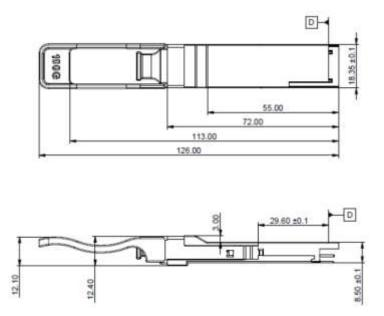
Note: Dimensions are in mm, All Dimensions are 0.2mm unless otherwise specified
