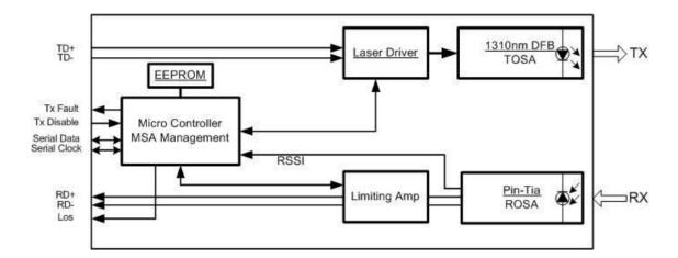
This 1310 nm DFB 10Gigabit SFP+ transceiver is designed to transmit and receive optical data over single mode optical fiber for link length 10km.
